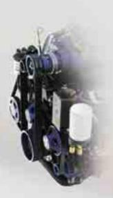
A one-piece serpentine belt system requires less horsepower to drive the engine accessories, is easier to service, needs less maintenance and provides unsurpassed belt life.
